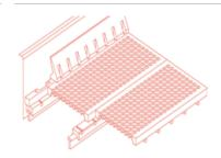
The supporting structure is made up of steel T-sections and a polyurethane adapter bar. The screen panels can then be simply inserted or replaced.
