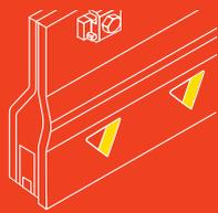
The Küper Cooling System features special openings to keep the blade from heating up.
