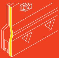
The Küper Wave Technology diverts snow across a curved profile for optimal removal. The snow is moved over the mounting elements without resistance.
